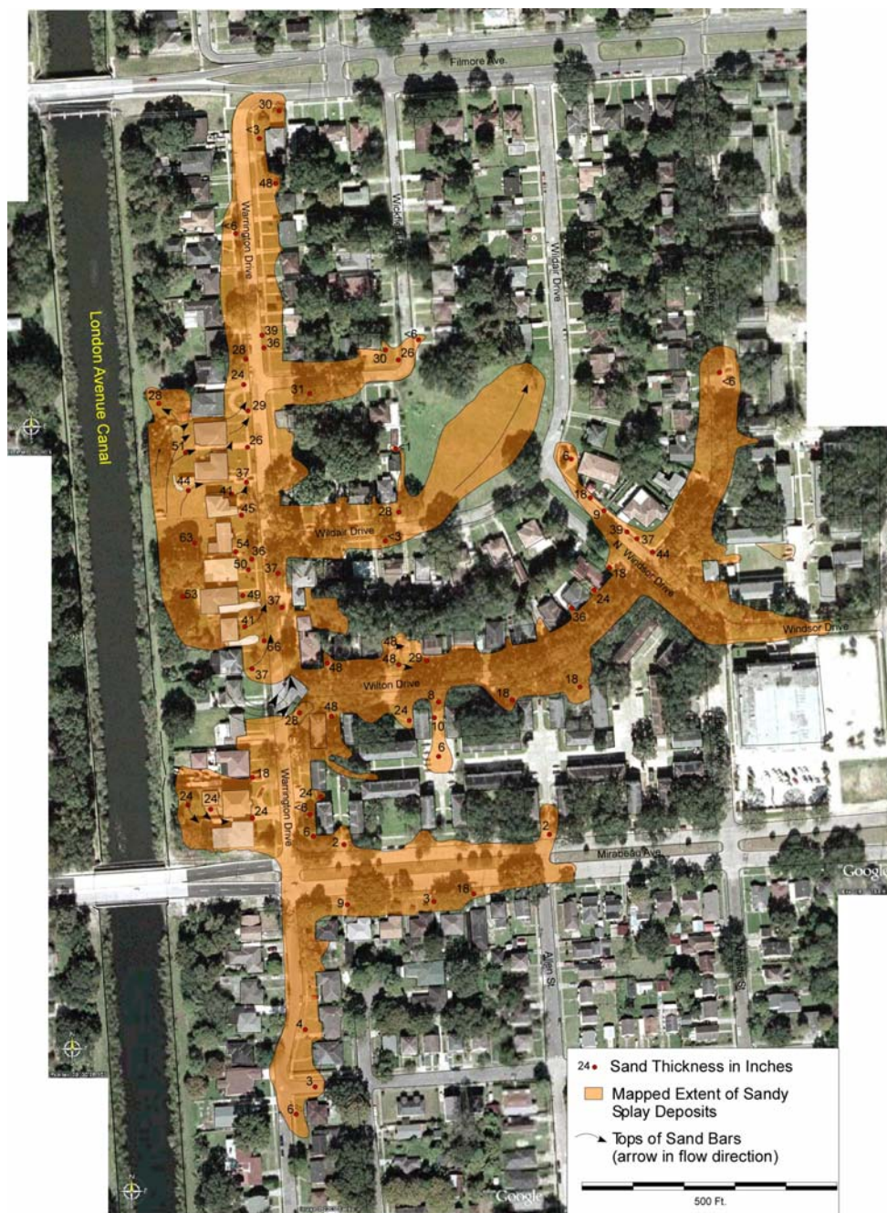
Figure 33. Preliminary map of sand deposits (by S. A. Nelson) from the Mirabeau Ave. breach on the London Ave. Canal. Underlying image is a composite from Google Earth.
