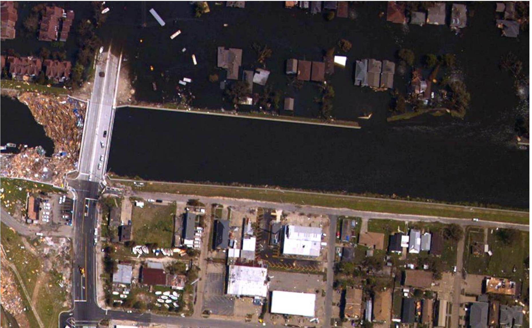
Figure 42. Air photograph of the area where the 17th Street Canal Levee was breached near Belaire Drive (Stop 8). Image acquired Aug. 31, 2005. Source: National Oceanic and Atmospheric Administration's National Geodetic Survey, Katrina Images - http://ngs.woc.noaa.gov/katrina/
