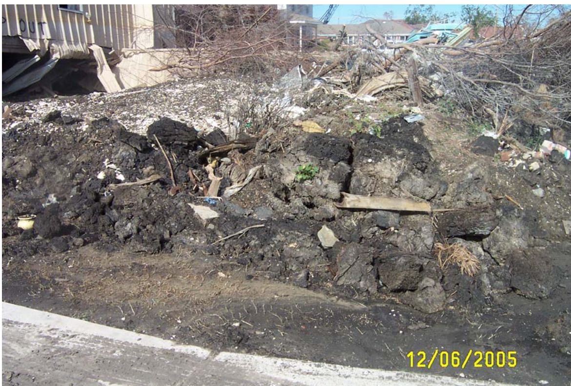
Figure 46. Blocks of Peat along Belaire Drive near the 17 th St. Canal levee breach
