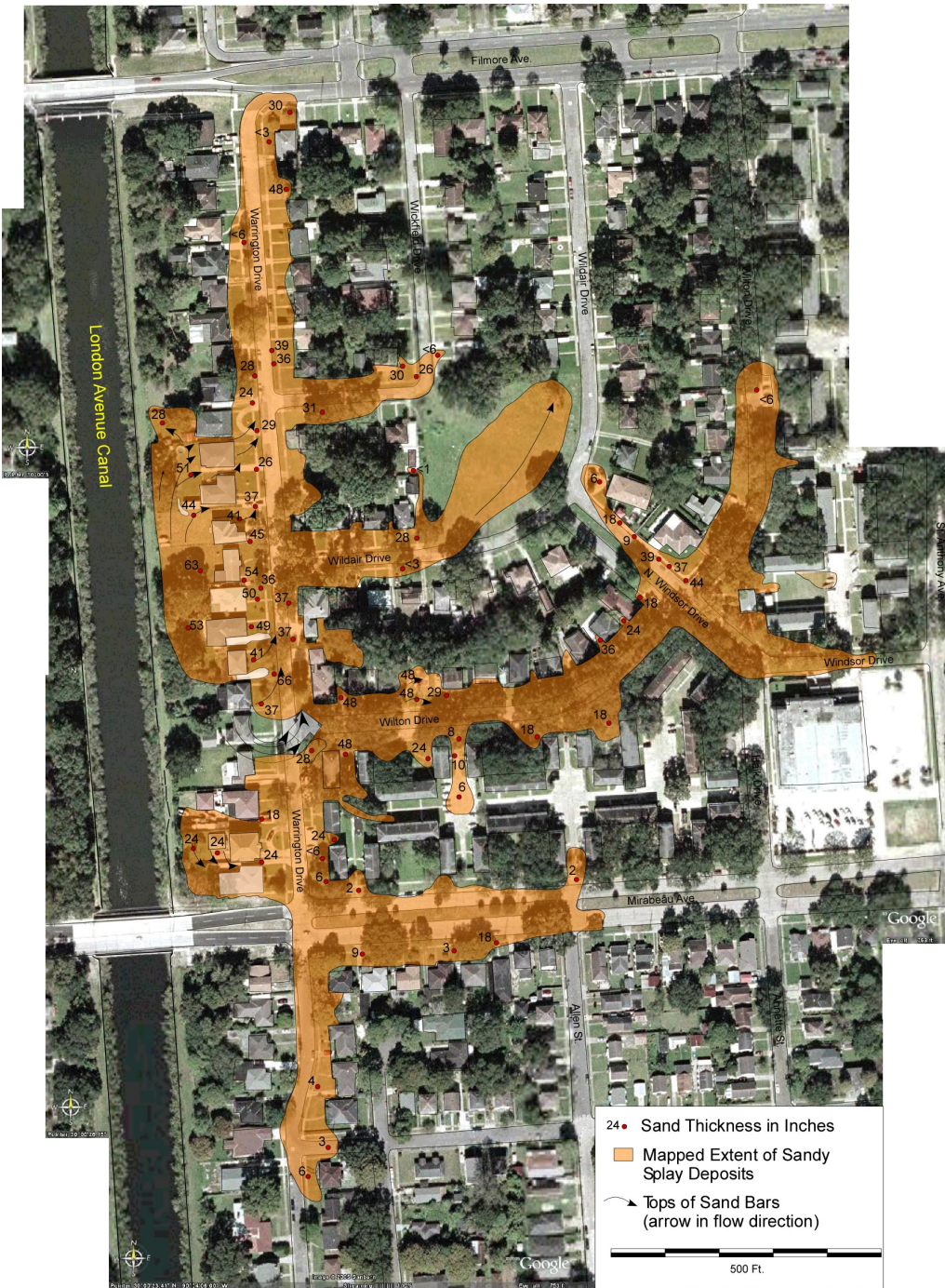
Figure 30. Preliminary map of sand deposits (by S. A. Nelson) from the Mirabeau Ave. Breach on the London Ave. Canal. Underlying image is a composite from Google Earth.
