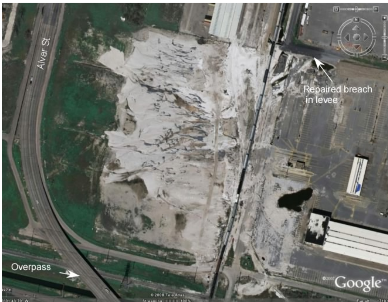
Figure 23. Google Image (acquired around May, 2006) of area near overpass to Alvar St. showing location of breached levee and deposits of shells (white material in center of image) that resulted from the breach. Industrial Canal is off the image to the right (east).
