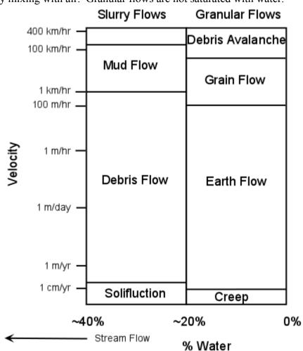
flows by mixing with air. Granular flows are not saturated with water.
