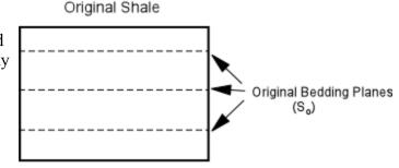
• *Slate* Slates form at low metamorphic grade by the growth of fine grained chlorite and clay minerals. The preferred orientation of these sheet silicates causes the rock to easily break planes parallel to the sheet silicates, causing a *slatey cleavage*.
