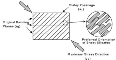
• *Schist* - The size of the mineral grains tends to enlarge with increasing grade of metamorphism. Eventually the rock develops a near planar foliation caused by the preferred orientation of sheet silicates (mainly biotite and muscovite). Quartz and feldspar grains, however show no preferred orientation. The irregular planar foliation at this stage is called *schistosity*
