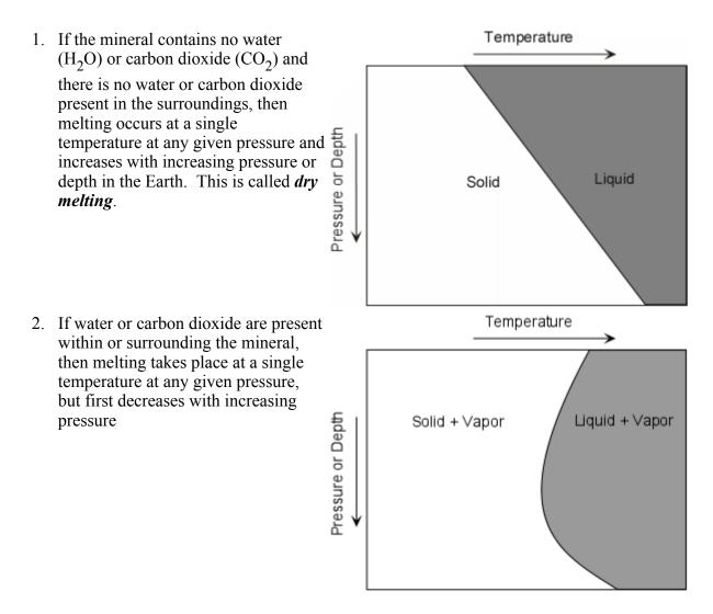
Since rocks are mixtures of minerals, they behave somewhat differently. Unlike minerals, rocks do not melt at a single temperature, but instead melt over a range of temperatures. Thus, it is possible to have partial melts, from which the liquid portion might be extracted to form magma. The two general cases are:
