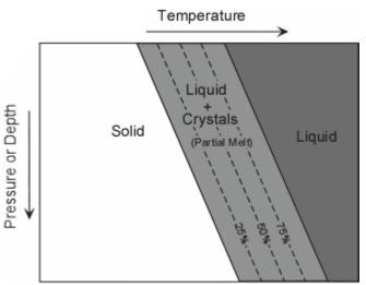
Temperature 2. Melting of wet rocks is similar to melting of wet minerals, except there is range of temperature range over which partial melting occurs. Again, Solid + Vapor Liquid Liquid + Vapor the temperature of beginning of Crystals Pressure or Depth melting first decreases with increasing pressure or depth, then at ;+ high pressure or depth the melting Vapor temperatures again begin to rise. (Partial Melt)
