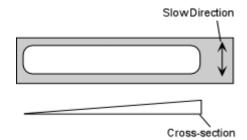
The wedge, like all compensators usually has its slow direction clearly marked, and is inserted into the microscope tube such that slow direction in the compensator is at a 45° angle to the polarizing direction. You will see a quartz wedge in the lab, but the microscopes we use do not have a slot that accommodates these older wedges. In today's economy, quartz wedges are too expensive to equip student microscopes with them.
