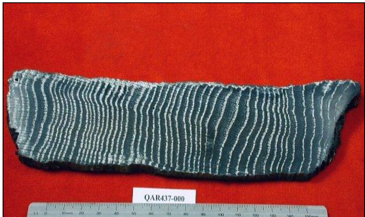
Figure 79, Quarter-sawn timber from Blackbeard’s Queen Anne’s Revenge, 1718
