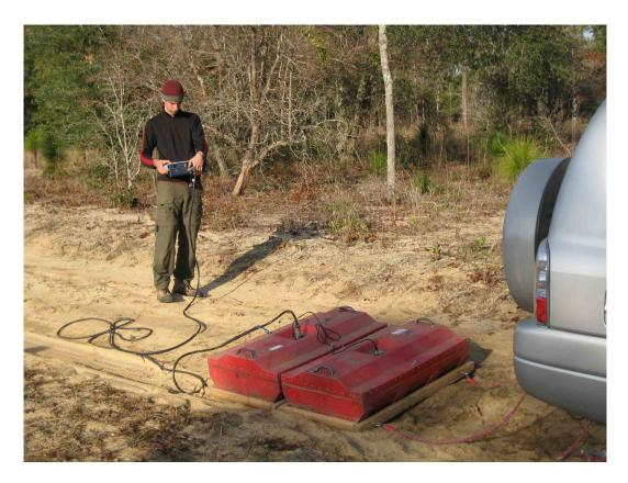
Figure S4: Configuration for the ground-penetrating radar survey. A 100 MHz bistatic radar antenna manufactured by Geophysical Survey Systems, Inc., was towed behind an automobile with an operator trailing the antenna and controlling the instrument with portable laptop.
