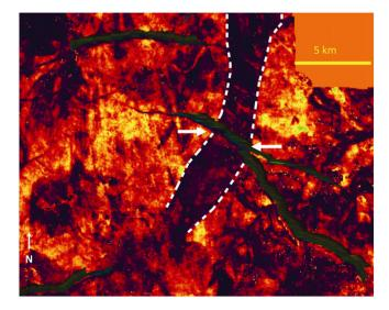
**Fig. 14.** Case B, a Miocene channel-belt system (dashed lines). View is from directly overhead with sweetness attribute shown. Hotter colors indicate higher sweetness. Arrows point to the fault with the channel-belt imaged as the dark, NNE–SSW aligned area between the two arrows.
