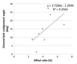
Fig. 21. Degree of channel-belt realignment by faults as a function of the fault offset ratio.
