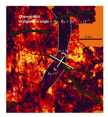
**Fig. 6.** Definition of channel-belt realignment angle measured at a fault crossing. The orientation of the channel-belt relative to the strike of the fault is measured both upstream,  $\Theta_{u}$ , and downstream,  $\Theta_{d}$ , of the structure. View (of channel-belt on a horizon slice in the seismic data) is from directly overhead; channel-belt is located in the NE portion of the survey approximately 1.5 km below the present surface.
