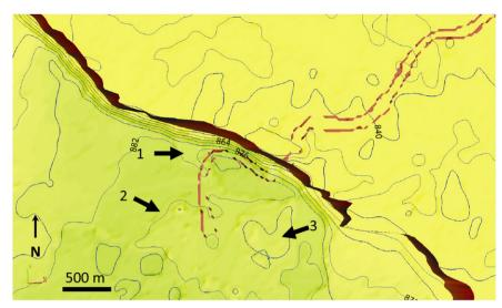
Fig. 12. Time-structure map of a surface that images the channel (map constructed from the seismic data). Numbered points indicate topographically high areas on the hanging wall of the mapped fault (shown here in brown striking northwest–southeast). Contour interval is 6 ms; yellows are high. View is from directly overhead.
