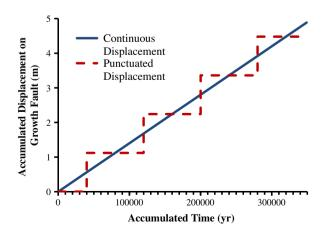
**Fig. 23.** Illustration of continuous fault displacement (blue line) with a rate of 0.014 mm/year versus punctuated displacement (red line) with an infrequently occurring ~1 m displacement.
