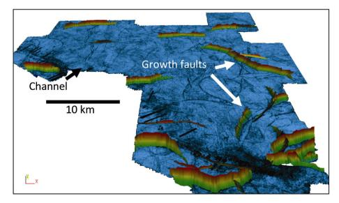
Fig. 2. A perspective view of a horizon slice in the seismic data (looking to the north) showing growth faults within the Miocene to Pliocene survey interval (hotter colors on growth faults indicate shallower depths). The blue surface shows outlines of several north-south oriented late Miocene fluvial systems.
