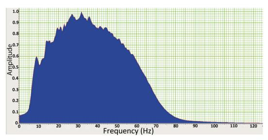
Fig. 5. Amplitude spectrum for the seismic volume from approximately 500 m to 2000 m below the present-day surface. Frequency content peaks at about 35 Hz and begins to decrease rapidly above 45 Hz.
