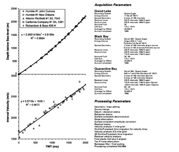
Fig. 4. The relationships between two-way travel time (TWT) and interval velocity and TWT and depth below the present-day surface derived from 5 checkshot wells in the study area (George, 2008). Seismic acquisition and processing parameters are also shown here.
