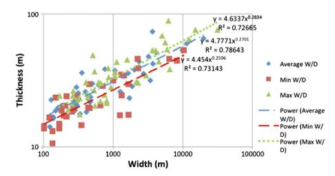
Fig. 9. Width (W) and depth (D) (i.e., channel or channel-belt thickness) average, minimum, and maximum values for forty-three fully mapped examples of fluvial stratigraphy in the seismic dataset.
