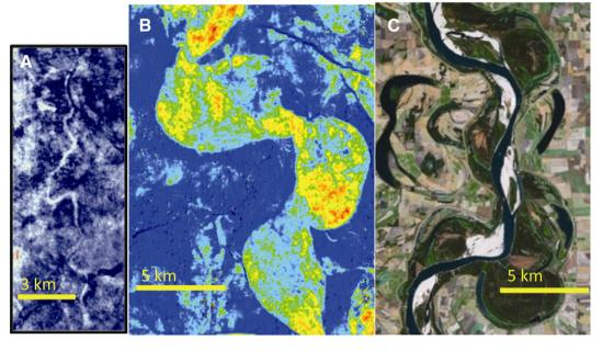
**Fig. 8.** Examples of channel and channel-belt fluvial styles. A) A north–south oriented channel approximately 200 m wide (from the seismic survey). B) A channel-belt ranging from approximately 2 to 4 km in width (from the seismic survey). C) A modern analog (the Mississippi River in southwestern Arkansas) for the formation of a channel-belt (satellite image from Google Earth®).
