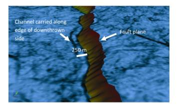
**Fig. 13.** Perspective view of a narrow channel aligned with the hanging wall of a growth fault for a distance exceeding 1 km. The growth fault is dipping to the left (red indicates shallowest level of the mapped fault). The channel is imaged here on a similarity attribute stratal slice from the seismic data.
