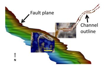
**Fig. 11.** A narrow Pliocene channel aligned with the downthrown side of a mapped fault. The two probes (rectangular boxes) show the channel planform as it appears in the amplitude volume. View is from directly overhead (2D view); hotter colors define shallower depths for the fault plane which is dipping to the left-hand side of the figure.
