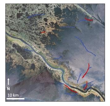
Fig. 3. Projections of fault planes overlain on a satellite photo; blue indicates a basinward fault dip and red indicates a landward dip. See Fig. 1 for regional location.
