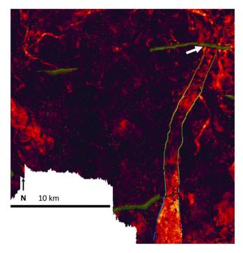
**Fig. 16.** Case D, a late Miocene channel-belt system (highlighted). View is from directly overhead on a map of the sweetness attribute. Hotter colors indicate higher sweetness values. The arrow points to where the fault intersects the channel-belt.
