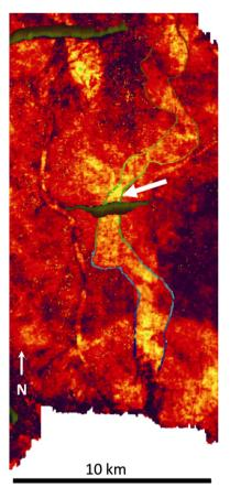
Fig. 15. Case C, a late Miocene channel-belt system (highlighted). View is from directly overhead with sweetness attribute shown. Hotter colors indicate higher values for the sweetness attribute. The arrow points to where the fault intersects the channel-belt.
