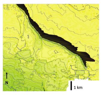
**Fig. 24.** Time map of surface around a fault (the fault is the dark shaded NW–SE oriented zone) with a 16 ms contour interval. The zone of enhanced, fault-created subsidence decreases to zero within ~500 m of the fault. Yellows indicate the shallowest parts of the mapped horizon.
