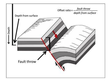
**Fig. 7.** Definition of offset ratio (from Gagliano, 2005). In the case where fault throw increases roughly linearly with depth, the offset ratio provides a simple way to compare the magnitude of faulting at different depths within the survey.
