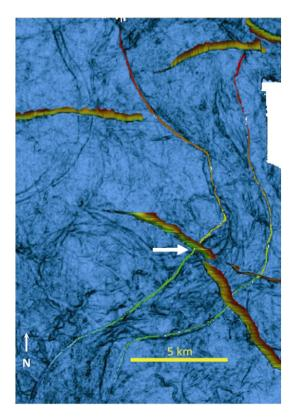
**Fig. 19.** Case G, a Pliocene channel-belt (highlighted). View is from directly overhead with similarity attribute shown. Darker colors indicate lower similarity. The arrow points to where the fault intersects the channel-belt.
