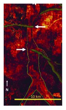
**Fig. 17.** Case E, a Mio-Pliocene channel-belt (highlighted). View is from directly overhead with sweetness attribute shown. Hotter colors indicate higher sweetness. The arrows point to where the faults intersect the channel-belt.
