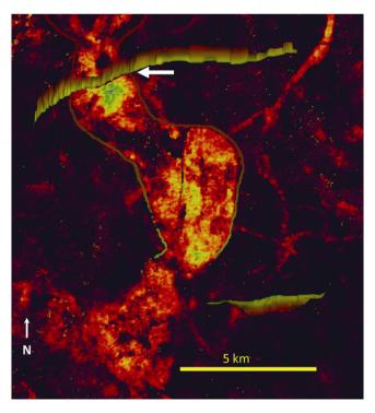
**Fig. 18.** Case F, a Mio-Pliocene channel-belt (highlighted). View is from directly overhead with sweetness attribute shown. Hotter colors indicate higher sweetness. The arrow points to where the fault intersects the channel-belt.
