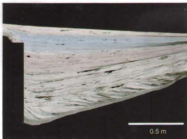
Fig. 6. A sliced dip section across the footwall and hangingwall in XES 08. The blue and top yellow layers were developed during the 4 th stage with two tectonically quiescent periods.
