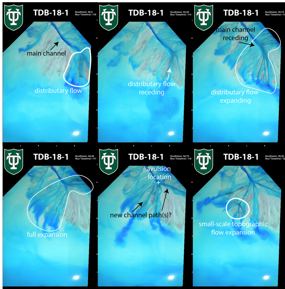
Figure B3. Topographic flow expansion from the control experiment displayed in hours 110, 113, 115, 117, 119, and 121. In this instance, it takes 11 h for the topographic flow expansion to occur.
