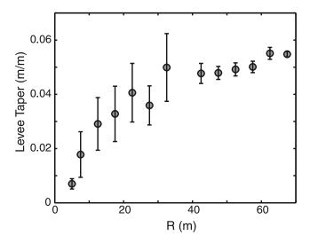
**Figure 7.** Change in the levee-deposit taper as a function of channel relief. Levee taper was defined from linear regression best fit lines through plots of average cumulative deposit thickness versus distance from channel. Taper was measured over a distance equivalent to two channel widths for each value of channel relief. Error bars are  $\pm 1$  standard deviation measured from variability in data defining deposit thickness versus distance from channel plots for each bin of channel relief.
