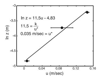
**Figure 10.** Estimation of model  $u^*$  obtained with best fit slope of ln *z* versus current velocity plot. Velocity measurements were obtained below the velocity maximum of each sample profile. Horizontal error bars are ±1 standard deviation calculated using all values for current velocity collected in each sampling volume;  $u^*$  value of the experimental flow events presented equals 0.035 m/s.
