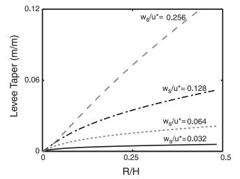
**Figure 16.** Model results documenting influence of sediment transport regime  $(w_s/u^*)$  on evolution of levee taper as a function of ratio between confining channel relief (R) and current thickness (H).
