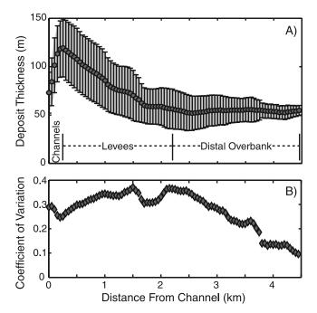
**Figure 6.** Change in deposit thickness as a function of shortest distance to a channel thalweg. (a) Mean thickness of deposit measured in bins spaced every 25 m from closest channel thalweg. Error bars represent  $\pm 1$  standard deviation of data in each bin. (b) Coefficient of variation for deposit thickness sample bins.
