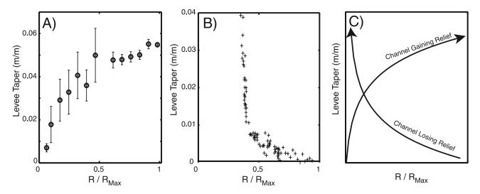
**Figure 14.** Evolution of levee tapers as a function of local channel relief divided by maximum channel relief for a give channel system. (a) Levee tapers measured for channel network offshore Brunei. (b) Levee tapers measured for laboratory experiment following flow 8. (c) Schematic diagram illustrating channel in levee taper for channel systems that gain relief through time and channel systems that loss relief through time.
