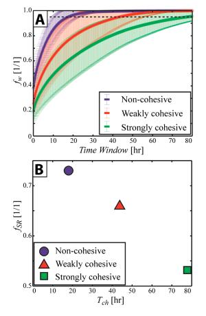
**Figure 3.** Data defining channel mobility and its implication on deltaic sediment retention. (a) Measurements of the increase in wet fraction on the fluvial surface as a function of time, used to estimate  $T_{ch}$ . Thick dashed lines represent time associated with wet fraction curve reaching 95% in each experiment. Error bars represent geometric standard deviation of each measurement. (b) Data defining relationship between  $T_{ch}$  and  $f_w$  in each experiment.
