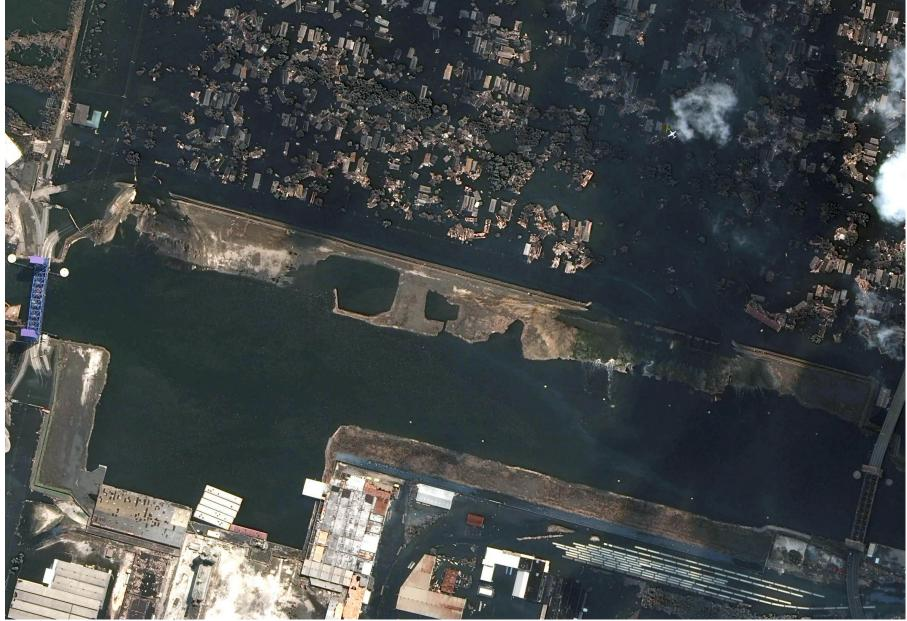
Figure 10. Air photograph of the area where the Industrial Canal Levee was breached to flood the Lower Ninth Ward. Image acquired Sept. 3, 2005 Source: National Oceanic and Atmospheric Administration's National Geodetic Survey, Katrina Images - <a href="http://ngs.woc.noaa.gov/katrina/">http://ngs.woc.noaa.gov/katrina/</a>
