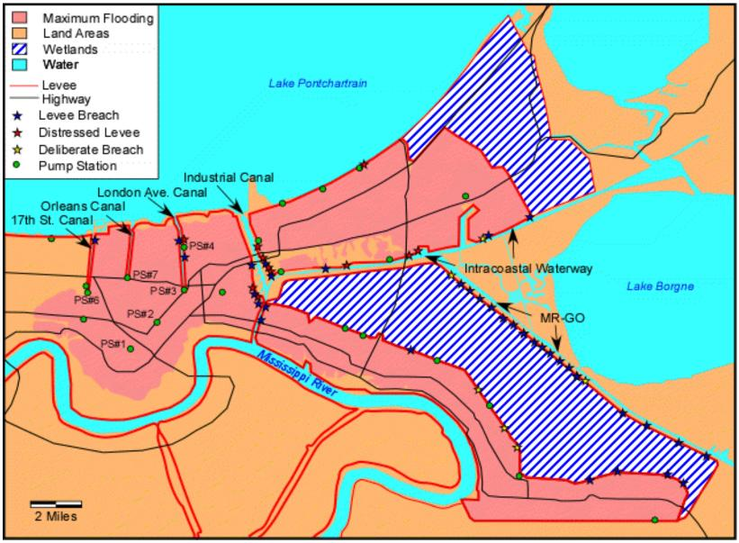
Figure 7. Map of maximum extent of floodwaters during Katrina modified and locations of breached levees after U.S. Army Corps of engineers-http://www.hq.usace.army.mil/cepa/katrina/pumps/pumps.html#New%20Orleans%20Pump%20Status and Seed et al. (2005).
