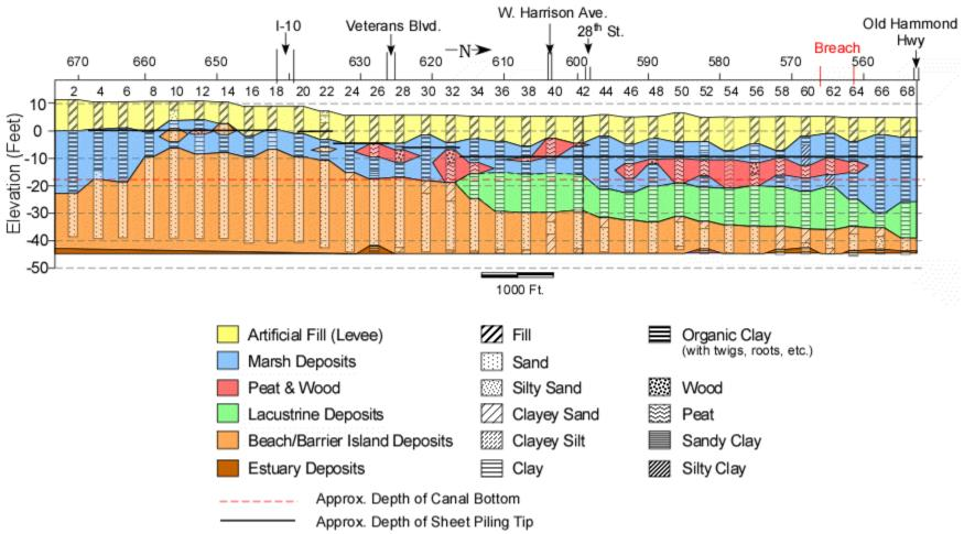
**Figure 28**. Geological cross-section along the eastern side of the 17<sup>th</sup> St. Canal (based on data in the U.S. Army Corps of Engineers design documents (1990). Notable in the cross-section is the peat layer that occurs in the area of the breach.
