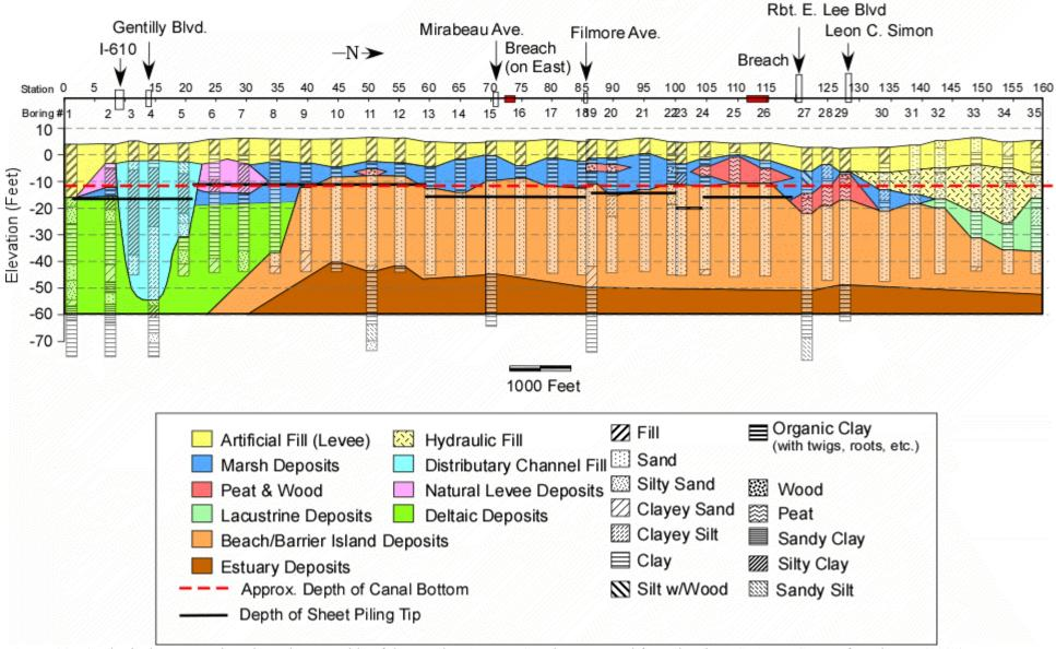
Figure 23. Geological cross-section along the west side of the London Avenue Canal constructed from data in U.S. Army Corps of Engineers (1989).
