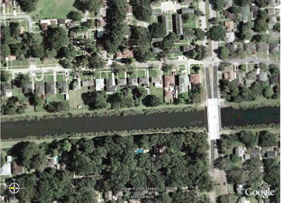
**Figure 14.** Satellite image of the area along the London Avenue Canal near Mirabeau Ave. and Warrington Drive (Stop 1), where the levee was later breached during Hurricane Katrina. (Source - Google Earth)
