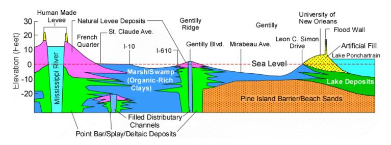
**Figure 6.** – Cross-section from the Mississippi River to Lake Pontchartrain showing Gentilly Ridge.
