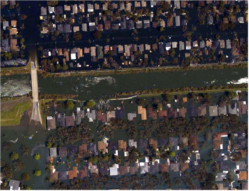
**Figure 22.** Air photograph of the area where the London Avenue Canal levee was breached near Robert E. Lee Ave. and Pratt Drive (Stop 2). Drive. Image acquired Aug. 31, 2005. Source: National Oceanic and Atmospheric Administration's National Geodetic Survey, Katrina Images - <a href="http://ngs.woc.noaa.gov/katrina/">http://ngs.woc.noaa.gov/katrina/</a>
