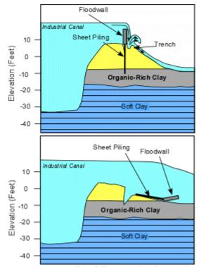
**Figure 13.** Possible failure mechanism at the Industrial Canal Levee breach in near the Lower 9<sup>th</sup> Ward.
