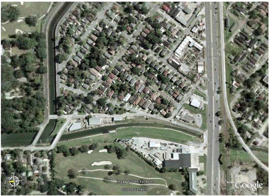
**Figure 33.** Satellite image of the area near the southern end of the 17th Street Canal near Old Metairie where water would enter Jefferson Parish from levee breaches in Orleans Parish during Hurricane Katrina (stop 5). (Source - Google Earth)
