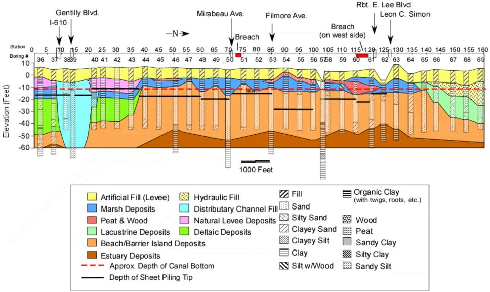
Figure 16. Geological cross-section along the east side of the London Avenue Canal constructed from data in U.S. Army Corps of Engineers (1989).
