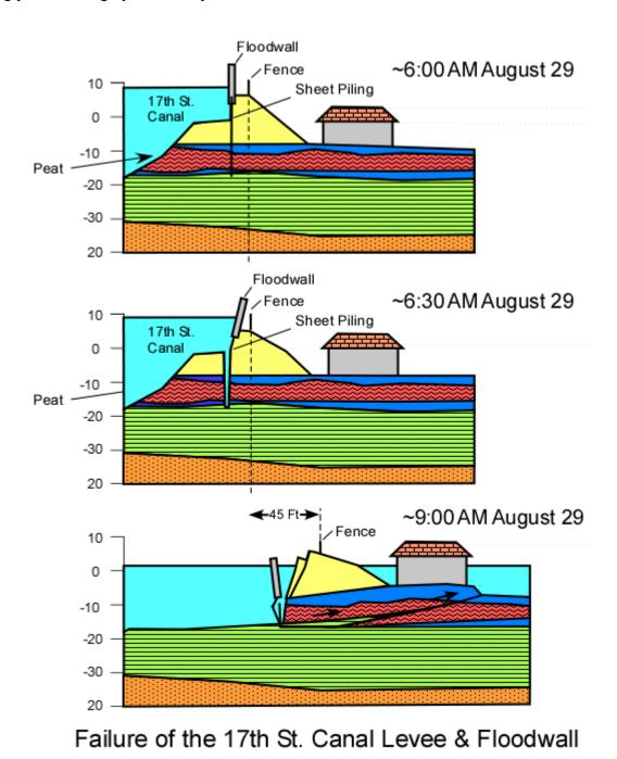
**Figure 29**. Diagrammatic cross sections across the 17 the Canal in the vicinity of the breach (based partially on a sketch in Seed and others [2005] and IPET (2006).
