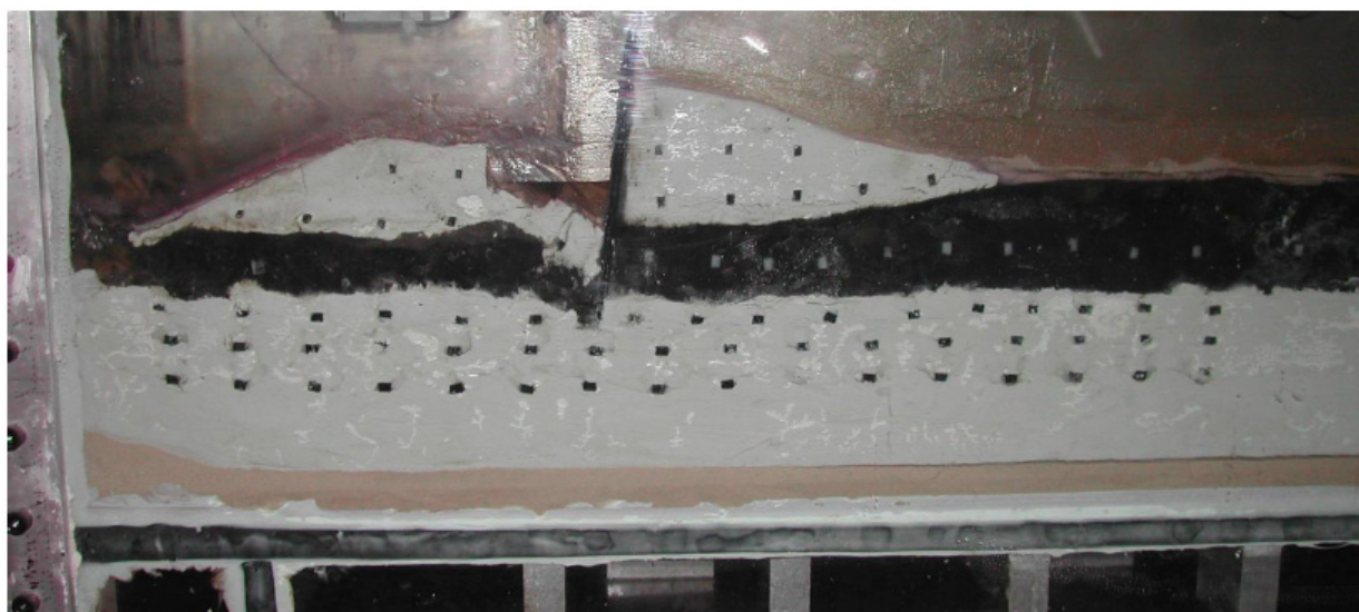
Figure 37. Photograph of failed levee and floodwall in IPET's scale model centrifuge experiment representing the 17 th St. Canal. The white at the top is clay and represents the levee. This overlies the dark peat layer, which in turn overlies another white clay layer meant to represent the estuary deposits beneath the peaty marsh deposits. Small rectangles were initially laid out in a rectangular grid and can be used to determine how much deformation has occurred during the experiment. (IPET, 2006).
