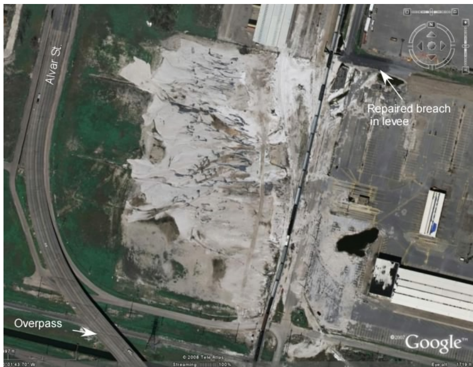
Figure 25. Google Earth Image (acquired around May, 2006) of area near overpass to Alvar St. (point A in Figure 1) showing location of breached levee and deposits of shells (white material in center of image) that resulted from the breach. Industrial Canal is off the image to the right (east).
