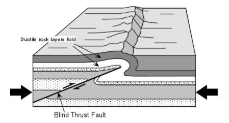
*Active Faults*- An active fault is one that has shown recent displacement and likely has the potential to produce earthquakes. Since faulting is part of the deformation process, ancient faults can be found anywhere that deformation has taken place in the past. Thus, not every fault one sees is necessarily an active fault.
