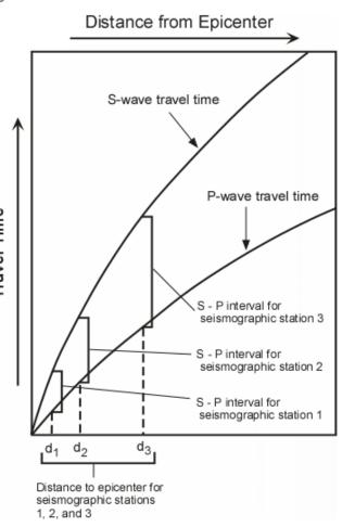
Thus the S-P interval tells us the distance to the epicenter from the seismographic station where the earthquake was recorded. Thus at each station we can draw a circle on a map that has a radius equal to the distance from the epicenter. Three such circles will intersect in a point that locates the epicenter of the earthquake.
