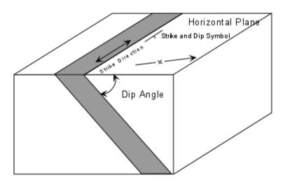
In recording strike and dip measurements on a geologic map, a symbol is used that has a long line oriented parallel to the compass direction of the strike. A short tick mark is placed in the center of the line on the side to which the inclined plane dips, and the angle of dip is recorded next to the strike and dip symbol. For beds with a  $90^{\circ}$  dip (vertical) the short line crosses the strike line, and for beds with no dip (horizontal) a circle with a cross inside is used.
