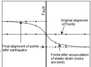
Friction between the blocks then keeps the fault from moving again until enough strain has accumulated to overcome the friction and generate another earthquake. Once a fault forms, it becomes a zone of weakness - so long as the tectonic stresses continue to be present more earthquakes are likely to occur on the fault. Thus faults move in spurts and this behavior is referred to as *Stick Slip*.
