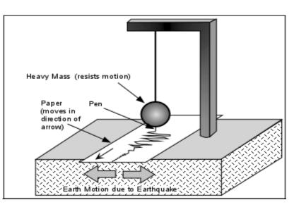
This is accomplished by isolating the recording device (like a pen) from the rest of the Earth using the principal of inertia. For example, if the pen is attached to a large mass suspended by a wire, the large mass moves less than the paper which is attached to the Earth, and on which the record of the vibrations is made. Modern instruments are digital and don't require the paper.
