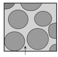
Water completely surrounds all grains and eliminates all grain to grain contact. Sediment flows like a fluid.
