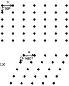
In the example to the right, the translation distances a and b are not equal and the translation angle is not  $90^{\circ}$ .
