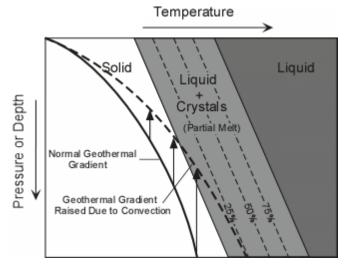
If the raised geothermal gradient becomes higher than the initial melting temperature at any pressure, then a partial melt will form. Liquid from this partial melt can be separated from the remaining crystals because, in general, liquids have a lower density than solids. Basaltic magmas appear to originate in this way.
