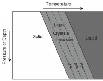
2. Melting of wet rocks is similar to melting of wet minerals, except there is range of temperature range over which partial melting occurs. Again, the temperature of beginning of melting first decreases with increasing pressure or depth, then at high pressure or depth the melting temperatures again begin to rise.
