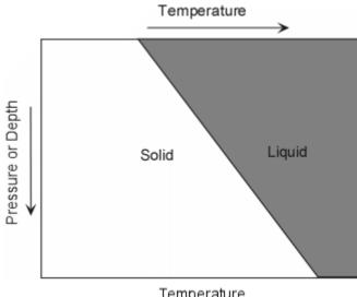
2. If water or carbon dioxide are present within or surrounding the mineral, then melting takes place at a single temperature at any given pressure, but first decreases with increasing pressure
