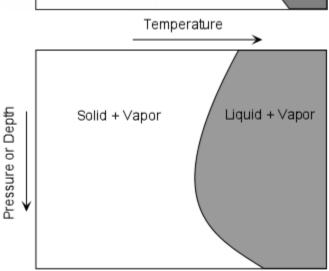
Since rocks are mixtures of minerals, they behave somewhat differently. Unlike minerals, rocks do not melt at a single temperature, but instead melt over a range of temperatures. Thus, it is possible to have partial melts, from which the liquid portion might be extracted to form magma. The two general cases are:
