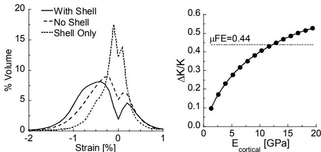
**Figure 3.** Histograms of maximum principal strains in the tissue for the three  $\mu$ FE models (left). Stiffness reduction vs. effective cortical shell modulus (right). The  $\mu$ FE value is shown with a dashed line.
