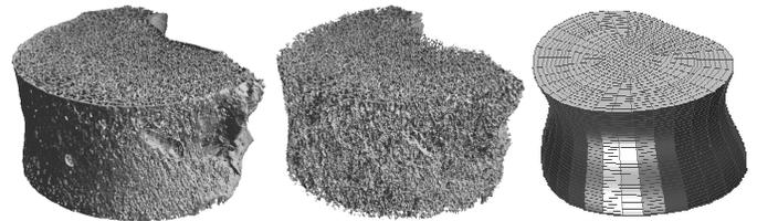
**Figure 2.** Vertebral body  $\mu$ FE model with (left) and without (center) the cortical shell. Geometry based generic model with shell (right).
