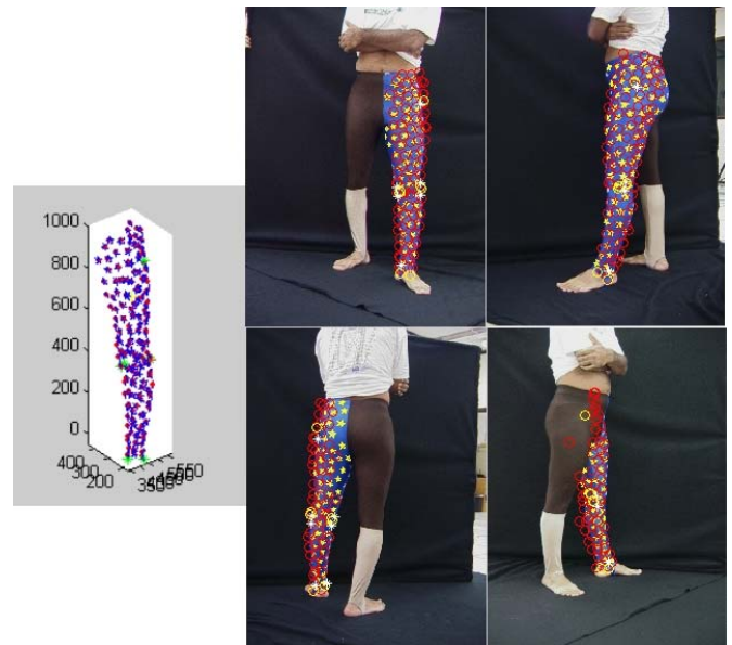
Figure 1. Subject wearing the spandex suit, viewed from four camera locations. Circles are the camera plane projection of the 3D model, shown on the left.
