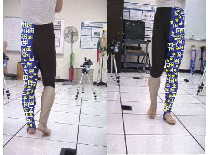
Figure 2. Results from two of six camera views. The subject data is shown in the star outlines. The back projection onto the camera planes are shown as squares.
