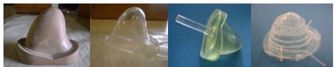
Figure 2. (From left to right): initial machined model; PMMA matrix; epoxy mould; final, reinforced prototype sac.
