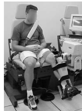
Figure 1: Subject test setup. The subject was seated in the Cybex chair. Lower limb is locked at 20° of flexion. Subject produced 1%, 2%, and 3% BW*Ht torque. KT-1000 provided relative motion between Femur and Tibia.
