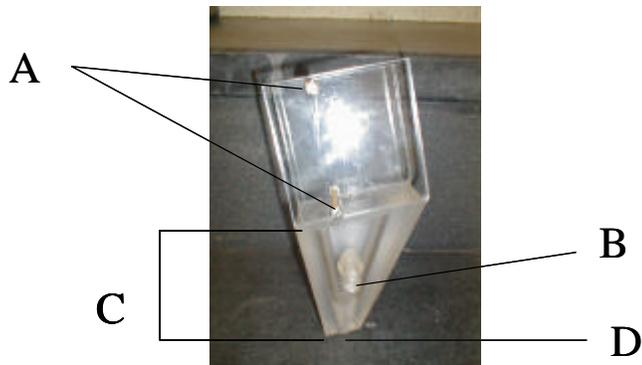
Figure 2: A) Screws that stabilize the laser to the acrylic casing. B) Nozzle where the aspirator tube is attached to produce a pressure. C) This internal area is hollow and sealed except for the narrow opening at D.
