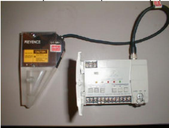
Figure 1: The LK-081 laser is held up by the acrylic casing on the left. The laser is also attached to the LK-2101 control on the right.
