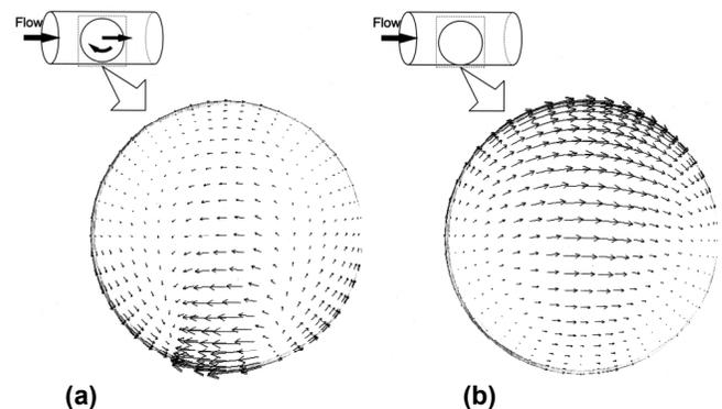
Figure 2. Shear stress distributions on the particle surface: (a) freely suspended sphere with  $a/R=0.8$  and  $c/R=0.15$ , and (b) adherent sphere with  $a/R=0.8$ . The scale of each arrow in (b) is one-third of that in (a).
