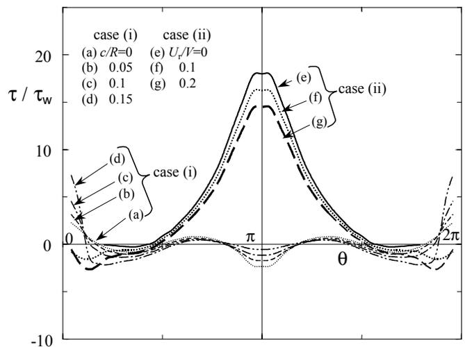
Figure 3. Shear stress distributions on the surface of a sphere along a circumference in the plane containing the center of the sphere and the vessel centerline.
