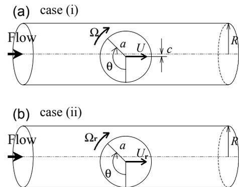
**Figure 1. (a) geometry for a freely suspended sphere in a vessel, and (b) geometry for a sphere adherent to or rolling along the vessel wall.**
