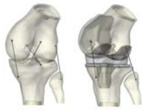
Figure 2. Kinematic model of the natural knee (left) and of the prosthetic one (right) at 60° flexion
