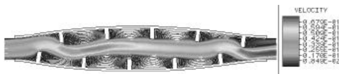
Figure 4. Velocity vector plot from CFD solution (legend unit in ms^{-1} ).
