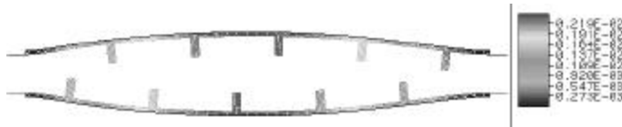
Figure 2. Nodal displacement of the cystic duct structure from CSD simulation (legend unit in m).
