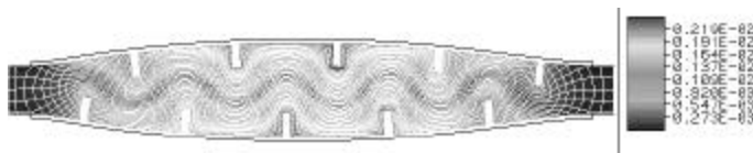
Figure 3. Nodal displacement from CMD remeshing scheme (legend unit in m).
