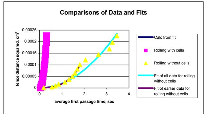
Figure 1. Rolling microsphere data and fits for all of the experiments.
