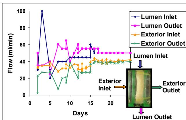
**Figure 3. Flow rate monitoring in the bioreactor** (flows are referenced with respect to the construct shown in the Figure)
