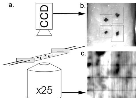
**Figure 2. a. Test apparatus layout: confocal objective, specimen under uniaxial strain, and a CCD camera. b. Computer display of the surface marker image captured by the CCD camera. c. Confocal image of the labelled collagen with the photobleached lines.**
