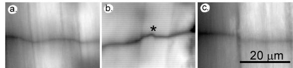
**Figure 5. High magnification confocal images at 4% strain a. a sloping line b. a mid-fiber dimple c. a dislocated line**
