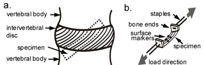
Figure 1. a. Orientation of the specimen preparation b. Prepared specimen and direction of applied load
