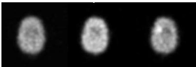
Figure 1. Interictal, Ictal (with 16% Perfusion Increase) and Ictal (with 200% Perfusion Increase), SPECT images of Brain Phantom on a GE Scanner, HAWKEYE
