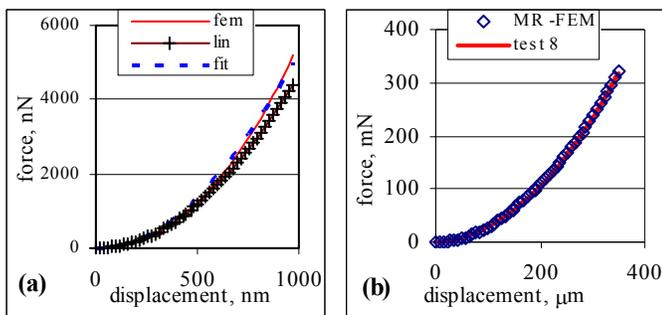
**Figure 1 (a). Force-displacement curves with  $C_2/C_1=1/8$  and  $E=4.8$ MPa for MR. (b) Comparison of predicted (MR-FEM) and measurements (test 8).**
