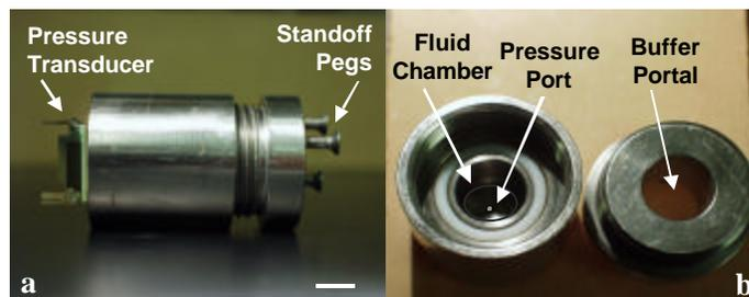
**Figure 1: Direct Membrane Osmometer (a) assembled device (b) fluid compartment, port for pressure transducer and access for buffer solution (scale bar=0.5 cm)**
