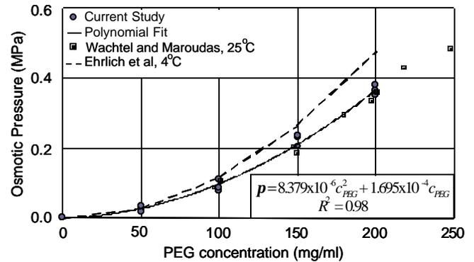
Figure 3: PEG calibration of osmotic pressure meter.
