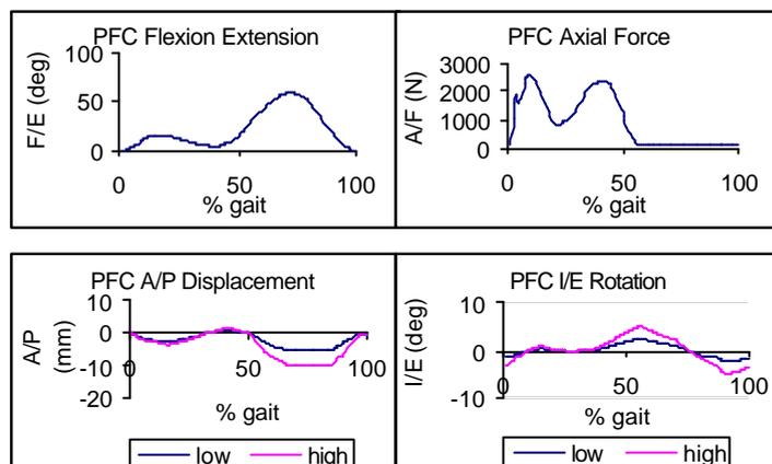
Figure 1. Flexion extension, axial force, A/P displacement and I/E rotation input parameters
