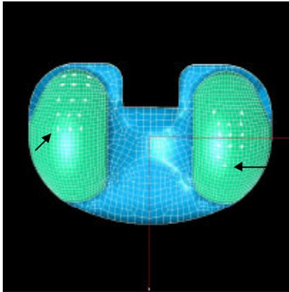
**Figure 2** Nodes selected from the polyethylene tibial tray – left hand side is medial, right hand side is lateral. Nodes indicated with an arrow have their wear paths included in the results section.
