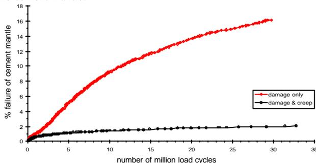
Figure 2. Element failure in cement, standard loadcase
