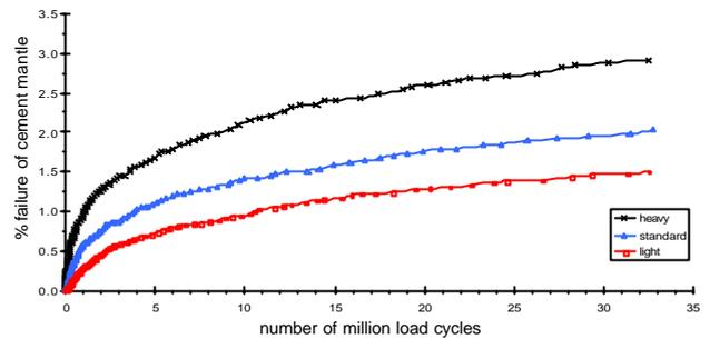
Figure 4. Element failure for different applied loads
