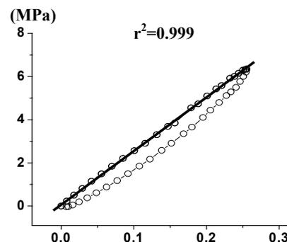
Figure 4 Stress-strain response for a typical specimen and linear curve fit of the loading data
