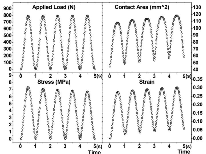
Figure 3 Dynamic response versus time for a typical specimen
