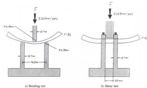
**Fig 1: Schematic Diagram of Bone Mechanical Testing [2]**
