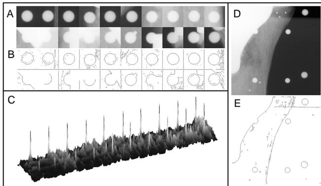
Figure 2: (A) A composite image of single markers; (B) The edge image for A; (C) The response for the convolution process; (D) A typical RSA image section; (E) The edge image for D
