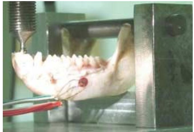
**Figure 1. Macromechanical test on mandible.**
