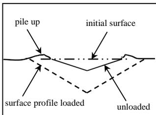
**Figure 1. Typical schematic of theoretical treatments.**
