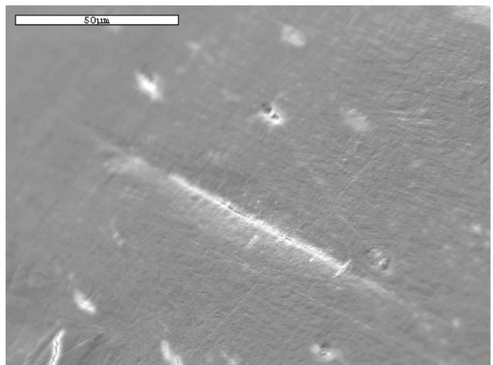
**Figure 4. Crack at microindentation apex.**
