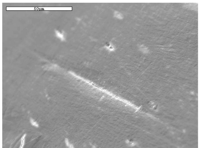
**Figure 4. Crack at microindentation apex.**
