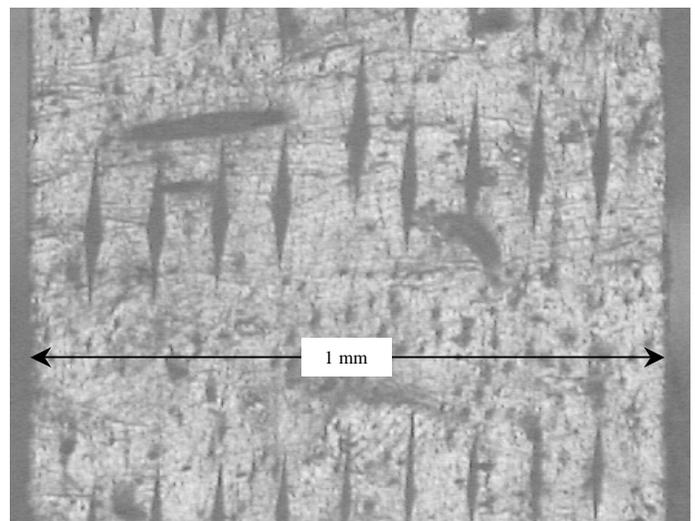
**Figure 2. Typical set of microindentations.**
