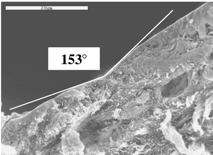
**Figure 3. Typical Knoop microindentation cross section for specimen indented dry**
