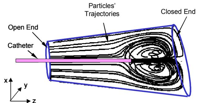
Numerical prediction of the trajectories of particles injected at a speed of 1 cm/s.
