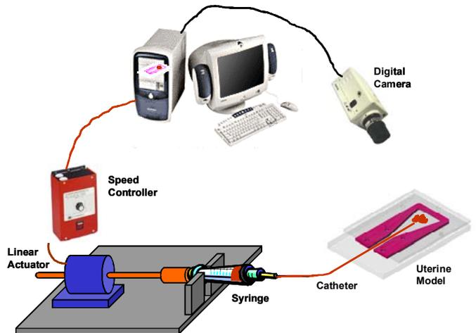
Figure 1. Scheme of setup for in vitro ET experiments.
