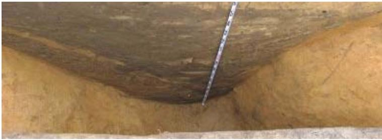
**Pictured above:** cross section of v-shaped trench
